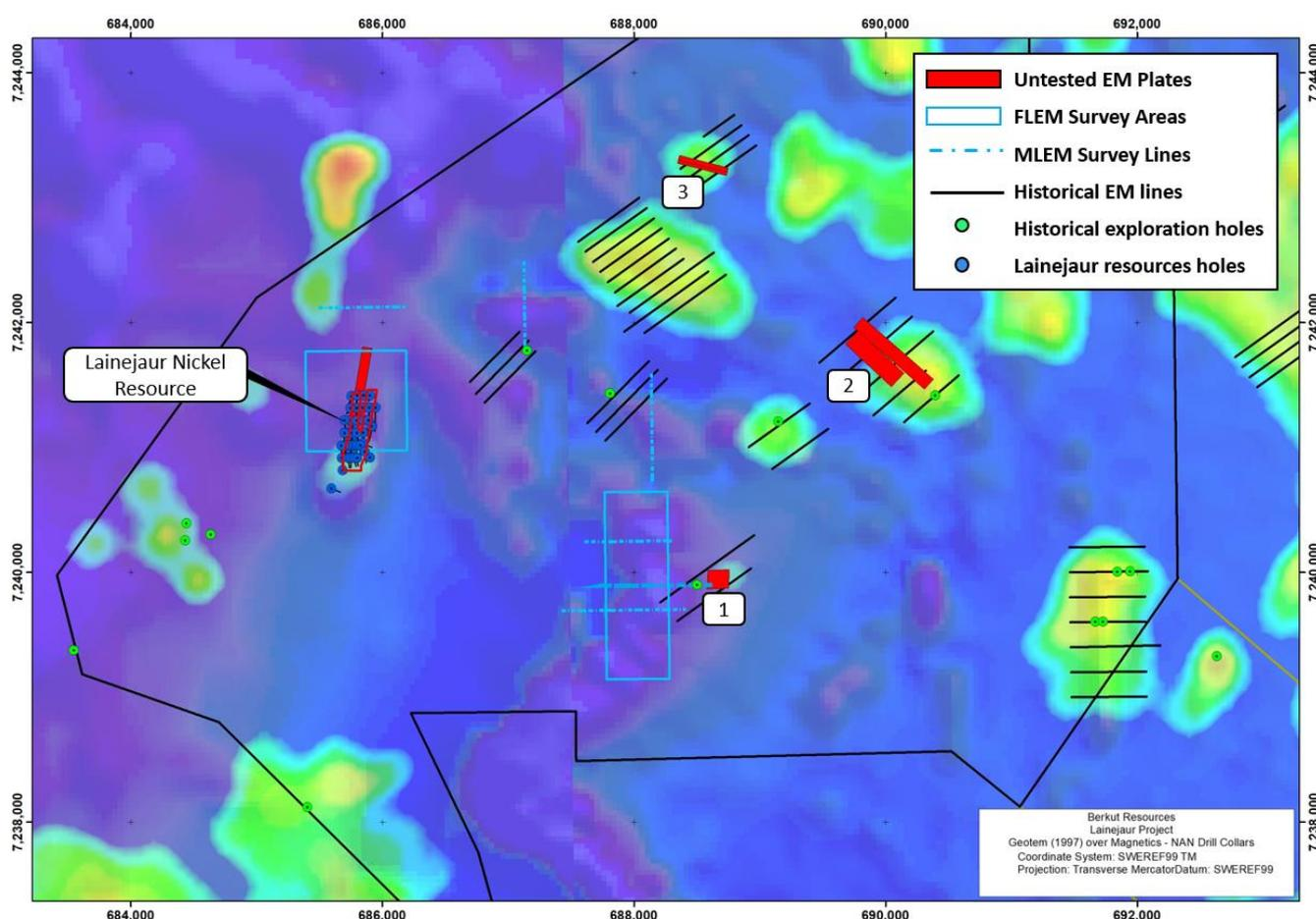
**Figure 4| Lainejaur Project Region: GEOTEM Time Constant (Tau) colour image with magnetic image as backdrop. Untested EM plates are shown as red polygons.**
